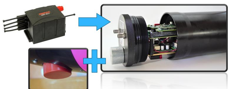
Cyprus Subsea redesigned the KM SIMRAD EK80 wideband transceiver (WBT) echosounder in order to fit in the M1 Seaglider payload bay. By reconfiguring the WBT electronics and placing them in a different geometrical configuration, these electronics fit into a cylindrical aluminium pressure housing. In addition to this reconfiguration, the design includes a 333 kHz single-beam transducer further streamlining the design by eliminating the need for one of the processing cards.
