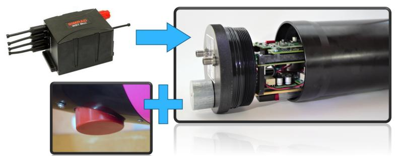
Cyprus Subsea redesigned the KM SIMRAD EK80 wideband transceiver (WBT) echosounder in order to fit in the M1 Seaglider payload bay. By reconfiguring the WBT electronics and placing them in a different geometrical configuration, these electronics fit into a cylindrical aluminium pressure housing. In addition to this reconfiguration, the design includes a 333 kHz or 200 kHz single-beam transducer further streamlining the design by eliminating the need for one of the processing cards.
