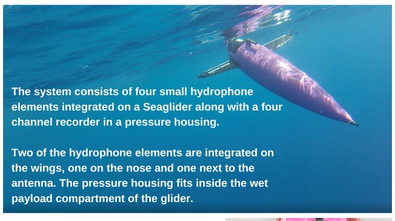
The system is currently capable of recording 128GB of acoustic data. Expansion to a few terabytes soon.
