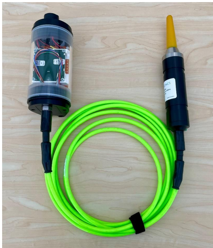
Figure 4: Bristlemouth with gListen Board connected to Ocean Sonics icListen Smart Hydrophone
